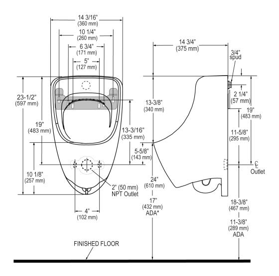
NOTE: ADA urinal rim height requirements allow all heights 17" and below. Sloan strongly recommends roughing in the drain to achieve a 16<sup>1</sup>/<sub>2</sub>" rim height or less to ensure compliance.
